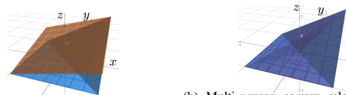
(a) Single ReLU polytope (shown in brown) gives looser upper bound for z . (b) Multi-neuron convex relaxation gives tighter upper bound for z (shown as two dark blue facets). Fig. 7. Comparison of convex relaxation for z = \text{ReLU}(x + y) (shown as bottom blue surface in (a)), where x, y \in [-1, 1] . Vertical axis is the z -axis.
