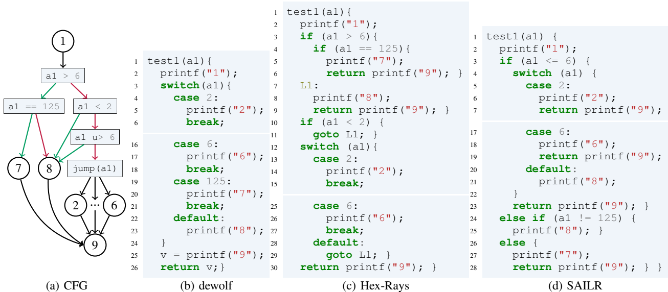
Figure 3: An exemplary CFG that does not obviously match a natural C-structure. While the pattern-independent approach dewolf recovers a natural C-Structure, namely a switch, as in the source code, Hex-Rays duplicates the return and uses a goto for the default, whereas SAILR duplicates the default and the return to avoid gotos. In contrast, Ghidra uses multiple gotos by not duplicating any code. All outputs have been standardized to highlight the structural differences.
