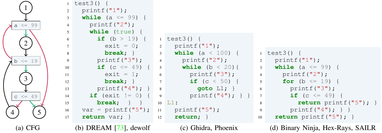
Figure 5: An exemplary CFG without a natural C-structure. Ghidra opted to use goto statements, whereas DREAM utilizes its multiple-exit restructuring, and Binary Ninja, Hex-Rays, and SAILR duplicate the return as well as the print-statement. All outputs have been standardized to highlight the structural differences.
